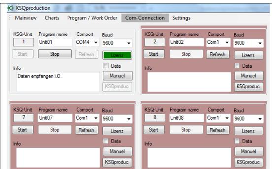
The menu Com-Connection is used to open, close and configure any com-connection to the KSQ-rectifier.
